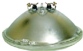
Screw-On Connections 24 Volts, 250W, 10.4 Amperes, 3000 Hrs + *, PEM #362-2005
